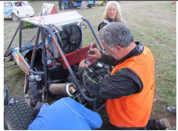
Class 8 – Bore & Stoke using specialist gauge kit.
