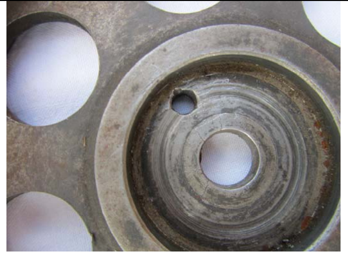
Lug hole does not have defined edges nor is circular.
